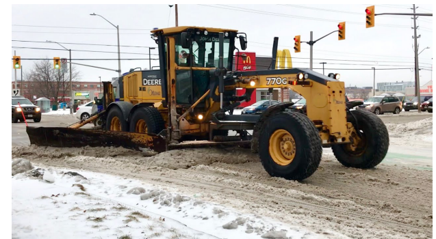
FIGURE 4.17 / LIMIT BUMP-OUTS TO INTERSECTIONS FOR EASE OF SNOW REMOVAL
